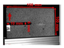
Figure 3 - Compact Tension Sample
