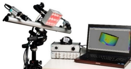
Figure 19 – Dantec Dynamics Q-400 DIC System with two cameras and illumination option
