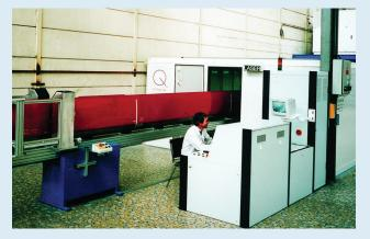
In preparation for the shearography process, the helicopter blade or other composite structure to be inspected is loaded into the vacuum chamber.
