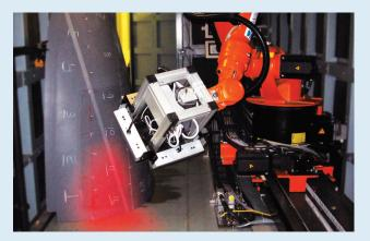
When the robot has confirmed the part's identification and all measurement locations, the operator initiates automated inspection at an initial surface area location, determined by the software program for the part. An unloaded image is taken first. Next, partial vacuum pressure is applied in the chamber and a loaded image is taken.
