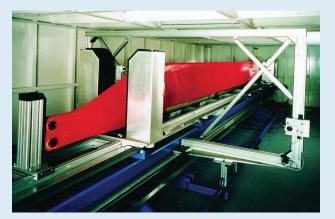
4 This process of capturing visual data for both unloaded and vacuumloaded images from part surface areas at program-determined locations is repeated down the entire length of the structure.
